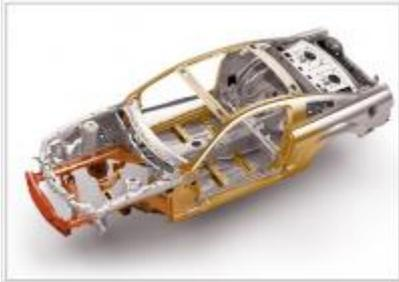
**FIGURA 13 SCOCCA PORTANTE IN LAMIERA D'ACCIAIO STAMPATA PER VETTURA FORD MUSTANG 2005**
